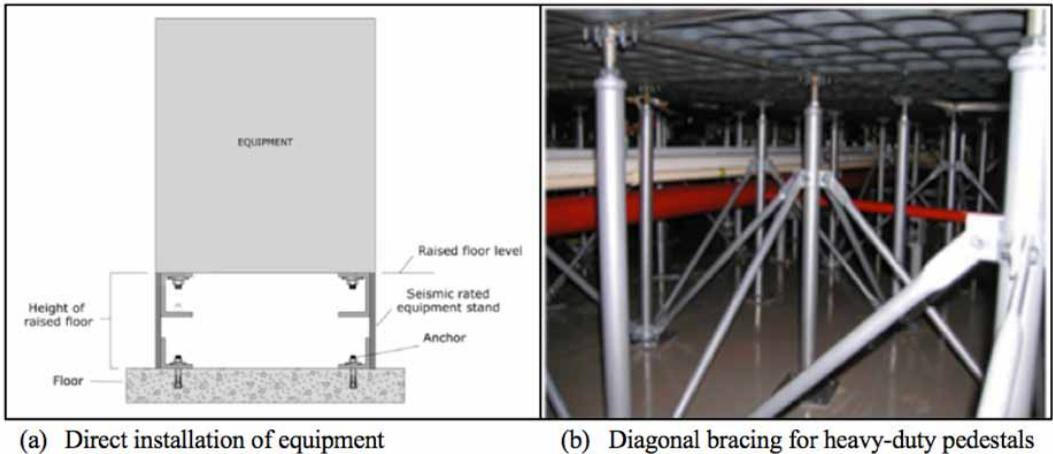
For seismic resilience of data centers, all raised floors shall comply with ASCE standards as follows:
